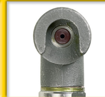
8. Check that seal is in correct position
