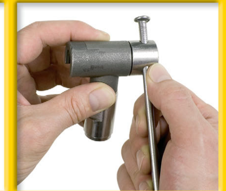
9. Tighten staple lock fitting with staple or nail
