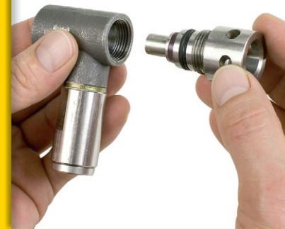
2. Remove staple lock fitting from nozzle housing
