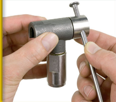
1. Loosen staple lock fitting with 6" nail
