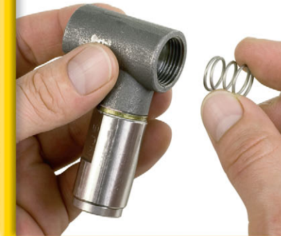
3. Remove spring from nozzle housing
