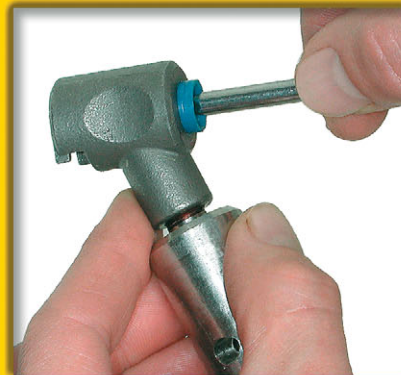
6. Push seal into nozzle
