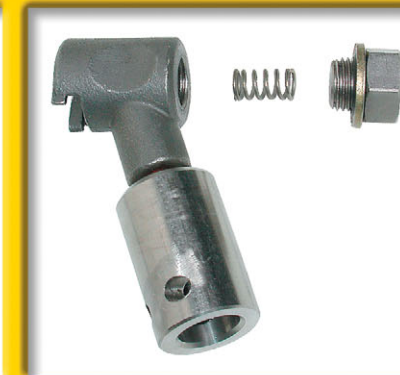
8. Replace spring and plug
