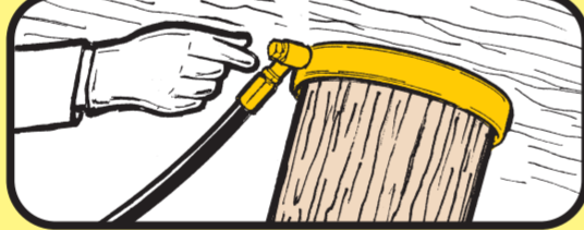
A. Check the relieving pressure daily (see "Pressure Setting" box). METHOD: Fit the pressure gauge to the nozzle at the end of the hose and pull the trigger.
