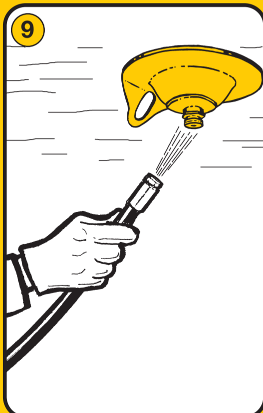
9. Remove the plastic cap from the valve. Check that the valve is clean and free of dirt and clean if required.
