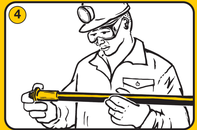
4. Check the RS-Bolt for any damage to the tube and the valve.
