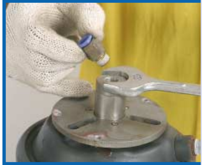
11. Using the No. 17 and 24 wrenches loosen and remove the push on fitting (AP1410S) and the flip flop cap (APFFCAP).
