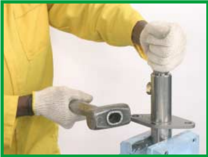
Then using the 4 pound hammer tighten the cylinder retaining plate (APCRPLT). Using a No. 30 wrench tighten the check valve body (APCVBOD).
