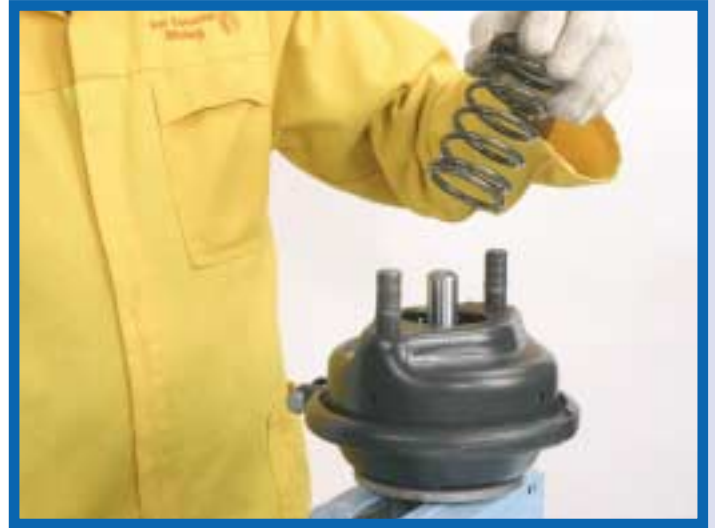
18. Now proceed to remove the cylinder phantom assembling (APCYLASS8) and the diaphragm's spring (APDSPR).
