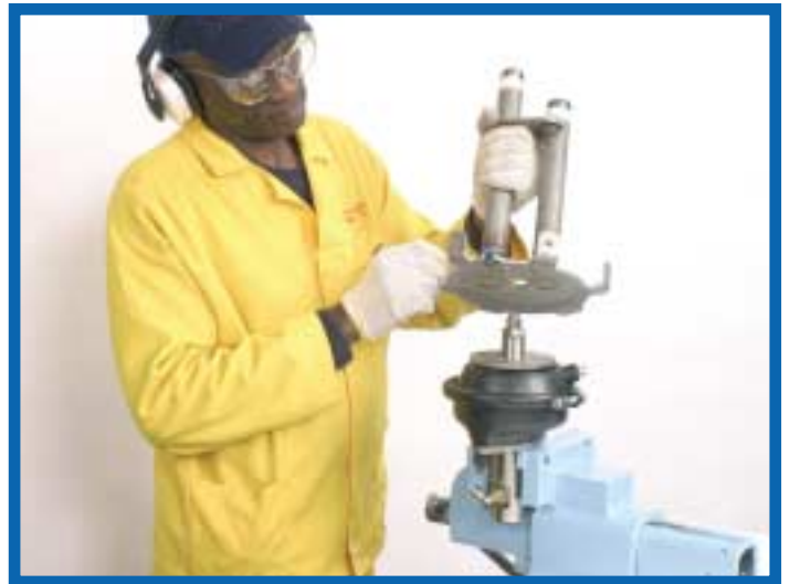
10. With the No. 5 Allen Key loosen the mounting plate screws (AP6X12) and remove the filters.
