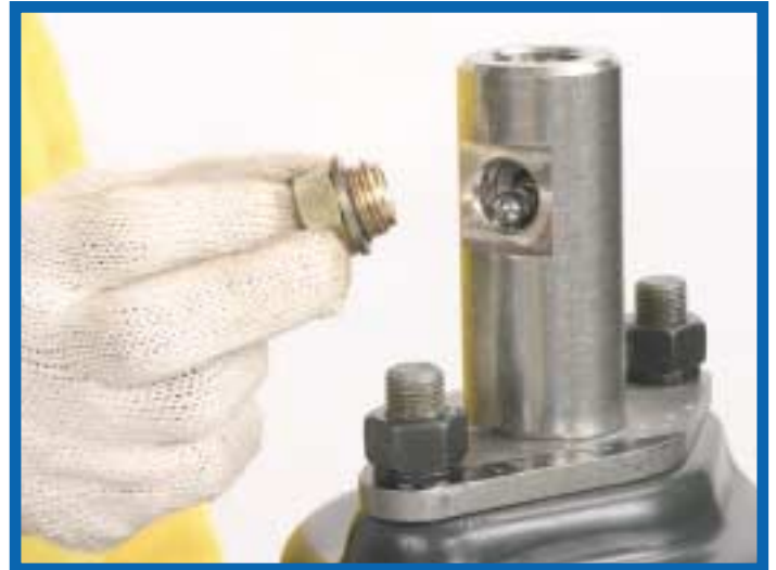
16. With the No. 24 wrench remove the check valve inlet (APCVINL), the Dowety washer (AP12DOW), the ball (HPBALL) and the spring (APCVSPR).
