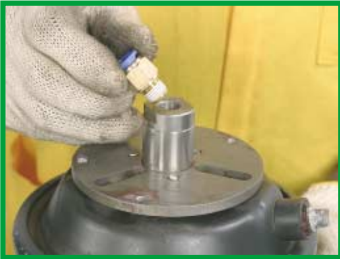
27. Wrap Teflon tape round the push on fitting thread (AP1410S) and tighten it with a No. 17 wrench.
