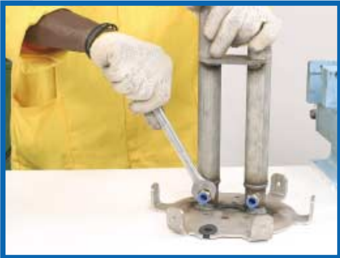
30. Using the No. 17 wrench loosen and remove the push on fittings (AP1410S) from the filter's assembly.
