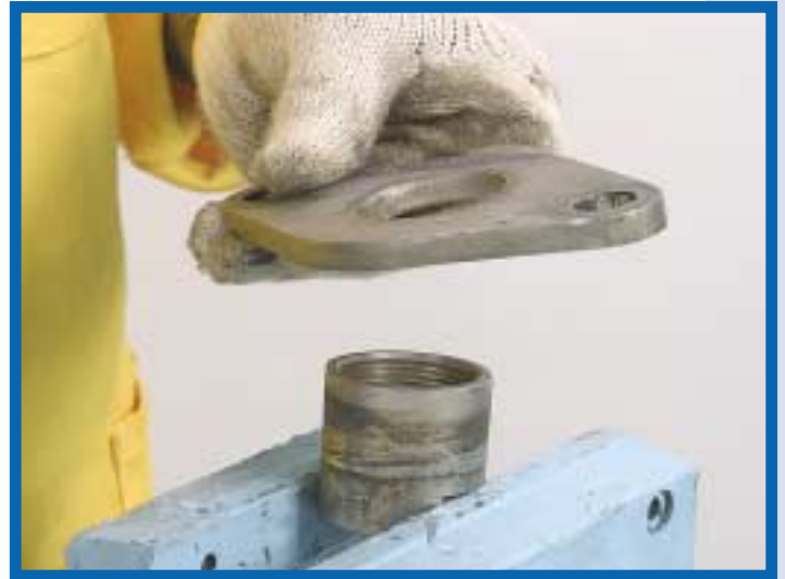
19. Place the cylinder in the bench vise and using the 4 pound hammer remove the cylinder retaining plate (APCRPLT) and the guide bush nut (APBNUT).
