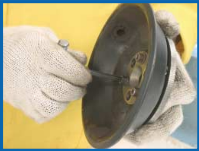
28. Using the No. 5 Allen Key loosen all three flip flop valve screws (AP6X16) of the actuator rear housing (APARH) and remove the exhaust plate (APEPLT), the flip flop body (APFFBOD) and the flip flop valve gasket (APFFVG).
