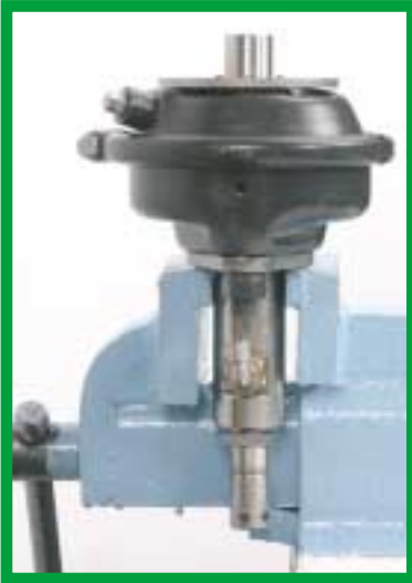
26. Place the actuator in the bench vise with cylinder facing down and put the flip flop cap (APFFCAP) in place, with its corresponding 'O' ring (APFFCO, a new one should there be a leak) and tighten it using a No. 24 wrench.
