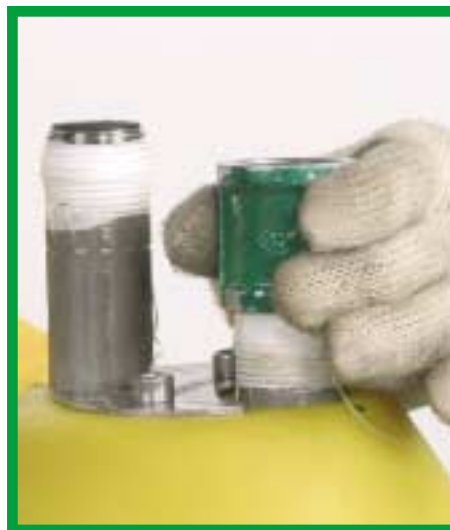
32. Use Teflon tape around the air and water inlets threads and install the appropriate size hose connectors.
