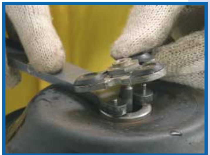
24. Using the wooden block supports (TK SJ) and the AP spanner (APSPANNER) remove the flip flop phantom assembly (APFFASS) of the diaphragm (APDIA) and the diaphragm plate (APDPLT).
