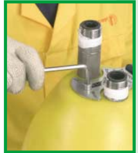
31. Place the pump in the bench vise and assemble the rear housing (APRHOU), the strap (APSTRAP) and tighten the two screws (HP8X16) with the No. 6 Allen Key.
