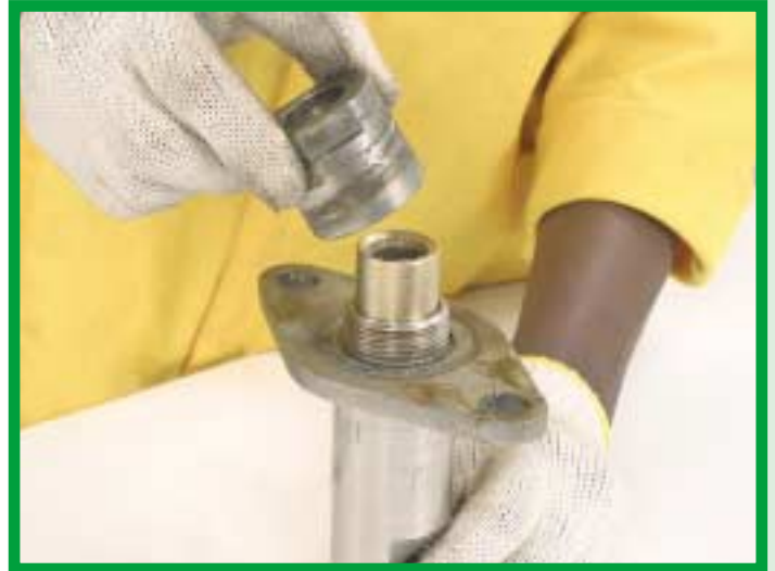
17. Assemble the cylinder (APCYL) with the cylinder plate (APCRPLT) and the guide bush nut (APBNUT).
