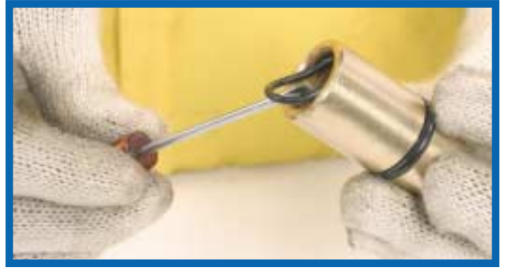
21. Using a small screwdriver remove all the seals and 'O' rings from the inside and outside of the piston guide bush (APGBUSH).
