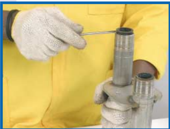
32. Use a screwdriver to pull up and remove the filters (APBAG).
