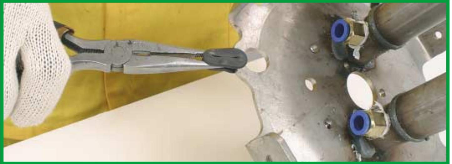
3. Using the pointed nose pliers insert the grommet (APGROM) in place.
