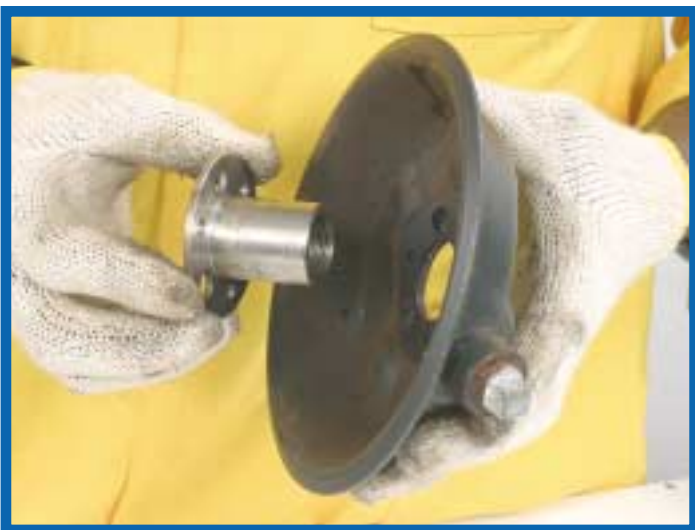
28. Using the No. 5 Allen Key loosen all three flip flop valve screws (AP6X16) of the actuator rear housing (APARH) and remove the exhaust plate (APEPLT), the flip flop body (APFFBOD) and the flip flop valve gasket (APFFVG).
