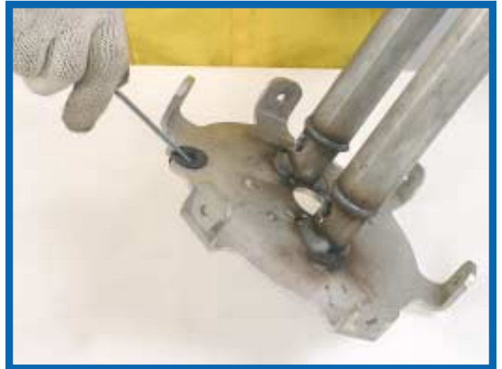
31. Use the small screwdriver to remove the grommet (APGROM) from the filter assembly.
