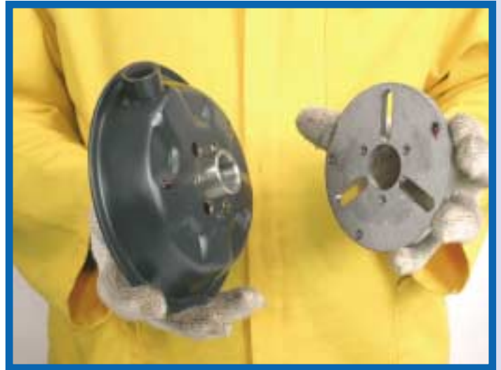
28. Using the No. 5 Allen Key loosen all three flip flop valve screws (AP6X16) of the actuator rear housing (APARH) and remove the exhaust plate (APEPLT), the flip flop body (APFFBOD) and the flip flop valve gasket (APFFVG).
