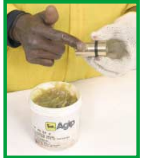
15. Apply lithium based multipurpose grease on the inside and outside the piston guide bush (APGBUSH).
