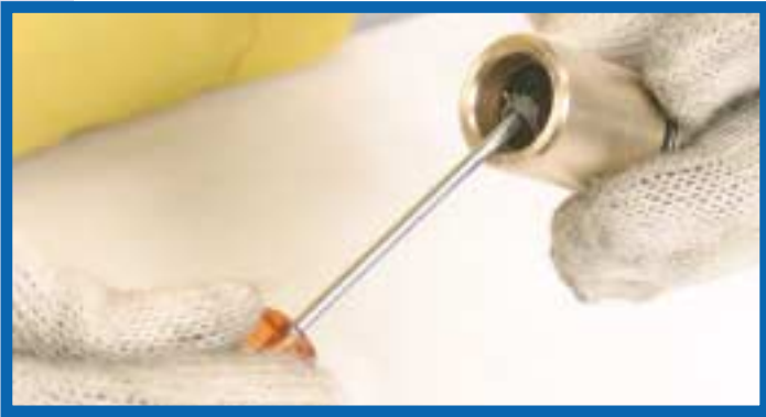
21. Using a small screwdriver remove all the seals and 'O' rings from the inside and outside of the piston guide bush (APGBUSH).
