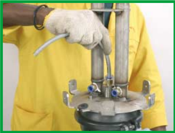
30. Then fix the water line and air line (AP10TU).
