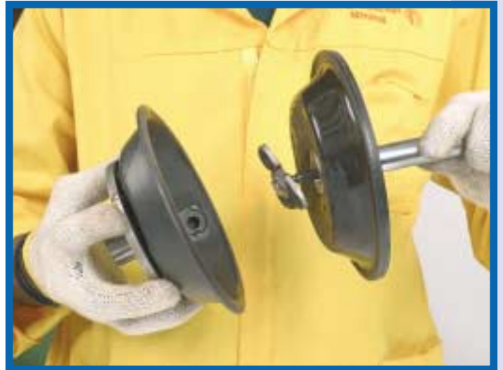
22. Using two No. 14 wrenches or the pneumatic tool with a No. 14 socket, unscrew the actuator housing screw and remove the clamp (APACLP).
