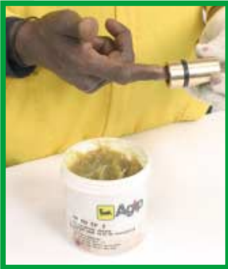
15. Apply lithium based multipurpose grease on the inside and outside the piston guide bush (APGBUSH).
