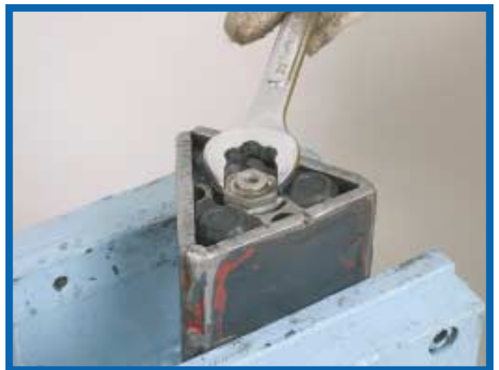
26. Place the flip flop valve plate (APFFVP) and the actuating pin (APAPIN) in the bench vise and using the No.19 wrench loosen the valve's nut (APFFVN).
