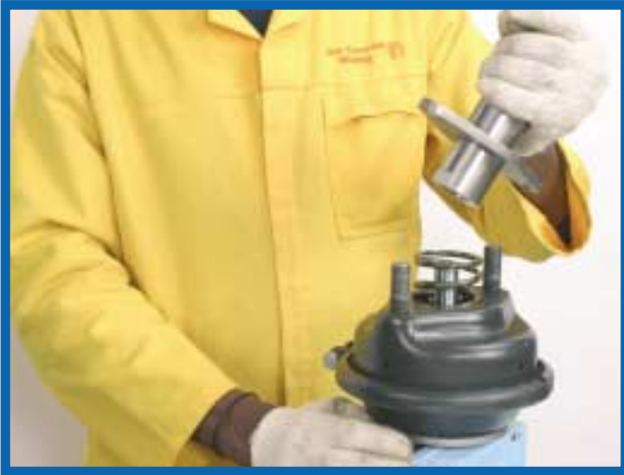
18. Now proceed to remove the cylinder phantom assembling (APCYLASS8) and the diaphragm's spring (APDSPR).
