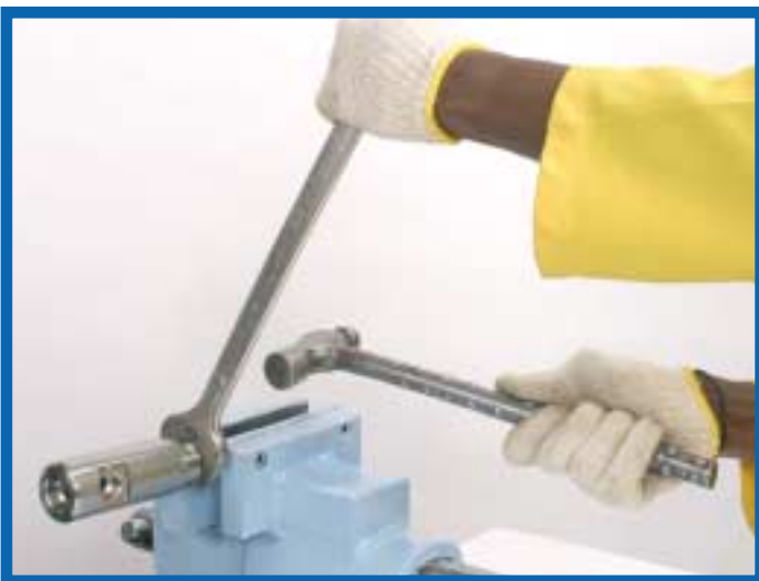
20. Place the cylinder assembling horizontally in the bench vise and using the No. 30 wrench and the hammer remove the piston guide bush (APGBUSH).
