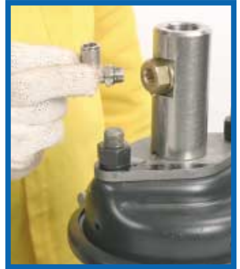
15. With the No. 16 wrench loosen the push fitting (AP1410E) of the cylinder assembling.
