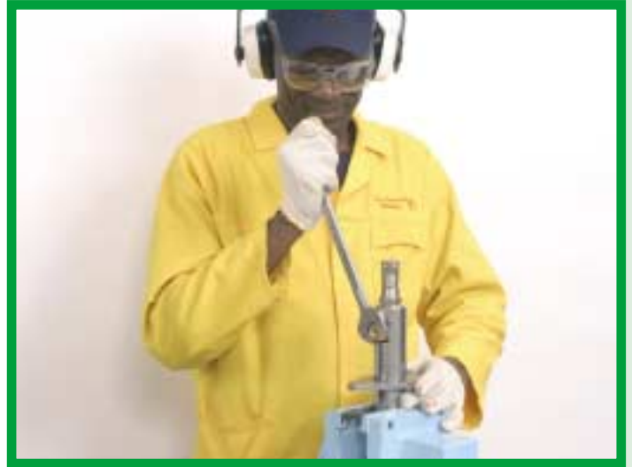
22. Using the No. 24 wrench tighten the check valve inlet (APCVINL).
