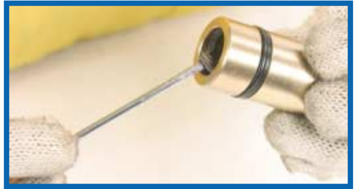
21. Using a small screwdriver remove all the seals and 'O' rings from the inside and outside of the piston guide bush (APGBUSH).
