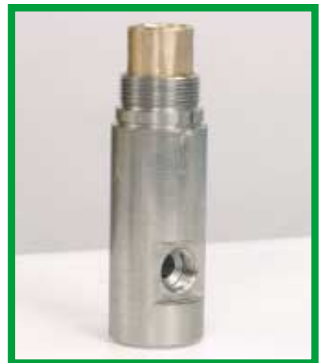
16. Insert the piston guide bush (APGBUSH) into the Cylinder (APCYL) ending with the flat back-up. Use a rubber mallet to tap in place.
