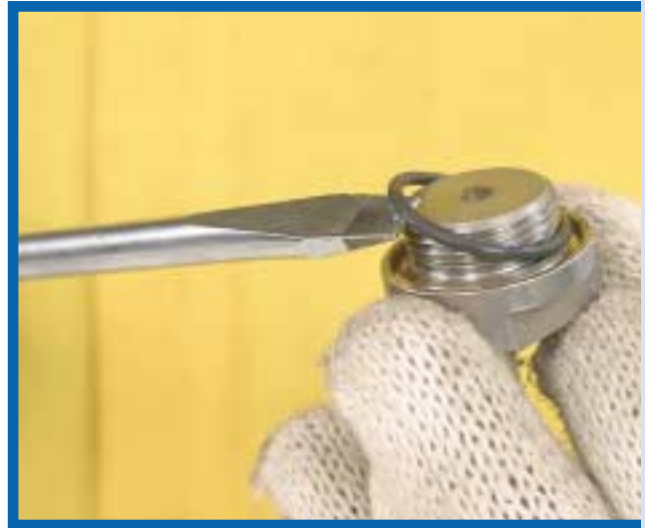
12. With the small screwdriver remove the flip flop cap 'O' ring (APFFCO).
