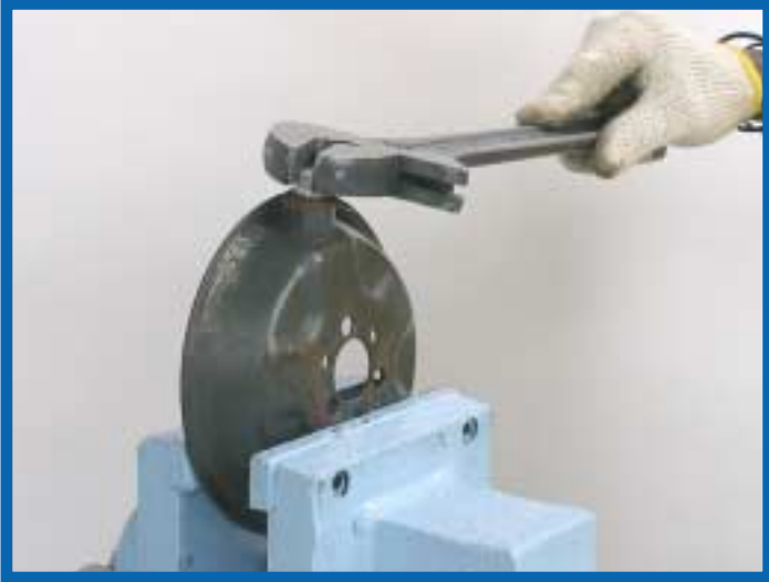
29. Place the actuator rear housing in the bench vise and using the 250mm/10" shifting spanner remove the actuator housing plug (AP38PL).
