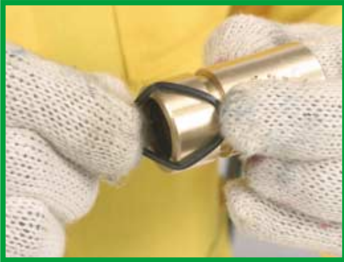
14. Do the same with the exterior flat back-up and the 'O' ring at the opposite end. The 'O' ring and the flat back up must be new.
