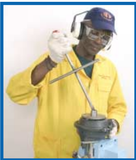
13. Using the 10mm x 300mm screwdriver loosen the popet screw from the flip flop inlet.
