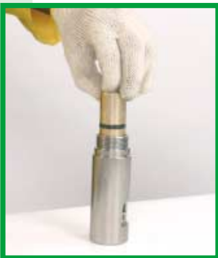
16. Insert the piston guide bush (APGBUSH) into the Cylinder (APCYL) ending with the flat back-up. Use a rubber mallet to tap in place.
