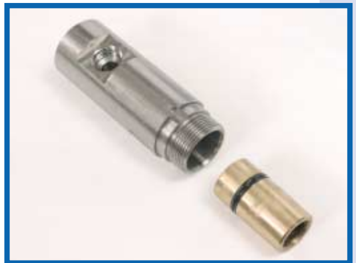
20. Place the cylinder assembling horizontally in the bench vise and using the No. 30 wrench and the hammer remove the piston guide bush (APGBUSH).
