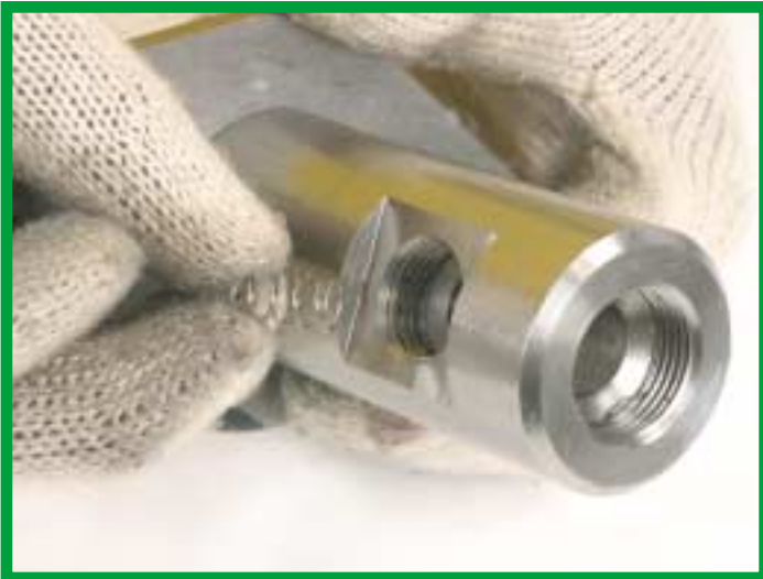
18. Fit the spring (APCVSPR) and the check valve ball (HPBALL) inside the cylinder. If the spring is damaged, it must be replaced.
