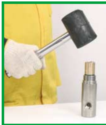
16. Insert the piston guide bush (APGBUSH) into the Cylinder (APCYL) ending with the flat back-up. Use a rubber mallet to tap in place.
