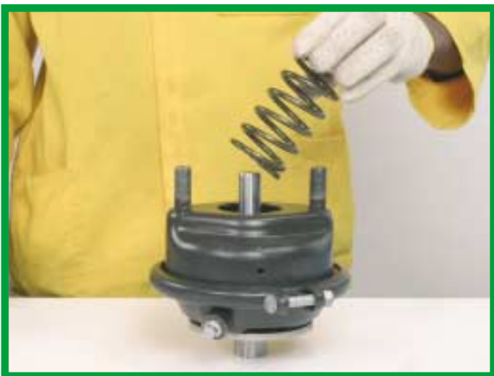
23. Insert the diaphragm spring (APDSPR) into the actuator assembly. Apply lithium based multipurpose grease to the actuator front housing screws and to the piston.
