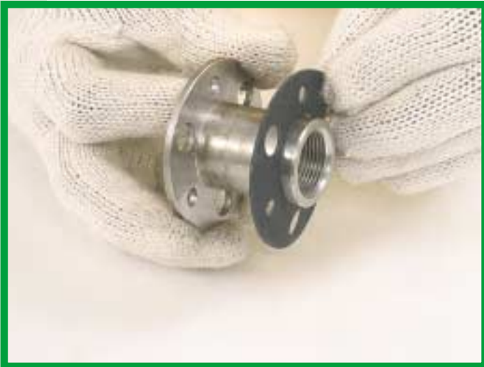
4. Assemble the actuator rear housing (APARH), the flip flop body (APFFBOD), if damaged, a new flip flop valve gasket (APFFVVG) and the exhaust plate (APEPLT) together. Align the set as shown in the red framed picture below.
