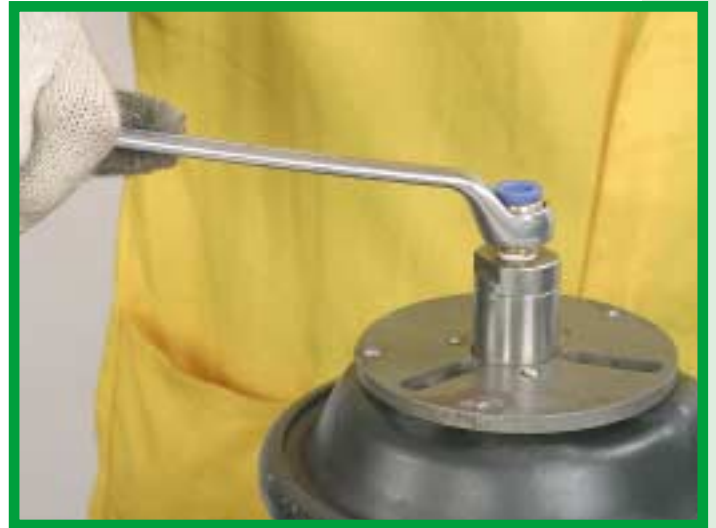
27. Wrap Teflon tape round the push on fitting thread (AP1410S) and tighten it with a No. 17 wrench.
