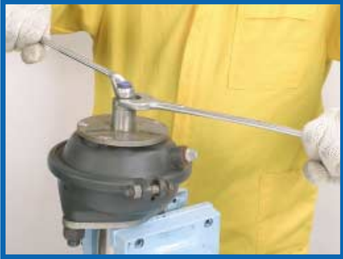
11. Using the No. 17 and 24 wrenches loosen and remove the push on fitting (AP1410S) and the flip flop cap (APFFCAP).
