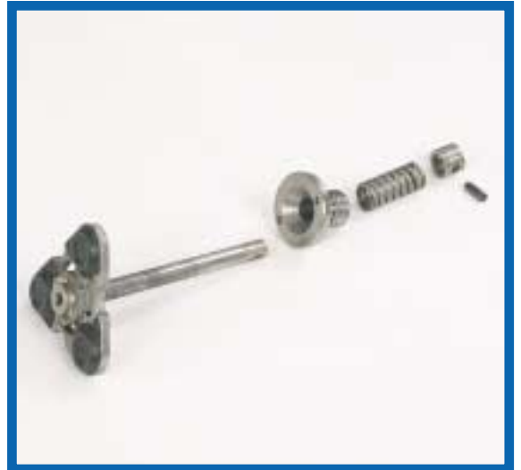
25. Place the flip flop phantom assembly (APFFASS) in the bench vise and using the punch and hammer remove the sellock pin (AP412SP) and disassemble the set.
