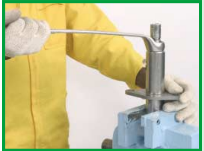
Then using the 4 pound hammer tighten the cylinder retaining plate (APCRPLT). Using a No. 30 wrench tighten the check valve body (APCVBOD).
