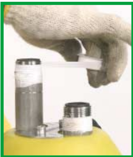
32. Use Teflon tape around the air and water inlets threads and install the appropriate size hose connectors.
