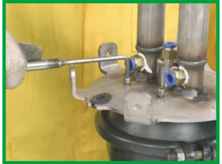
29. Fit the filters assembly, apply threadlock 3247 to the screw holes (AP6X12) and tighten with a No. 5 Allen Key.
