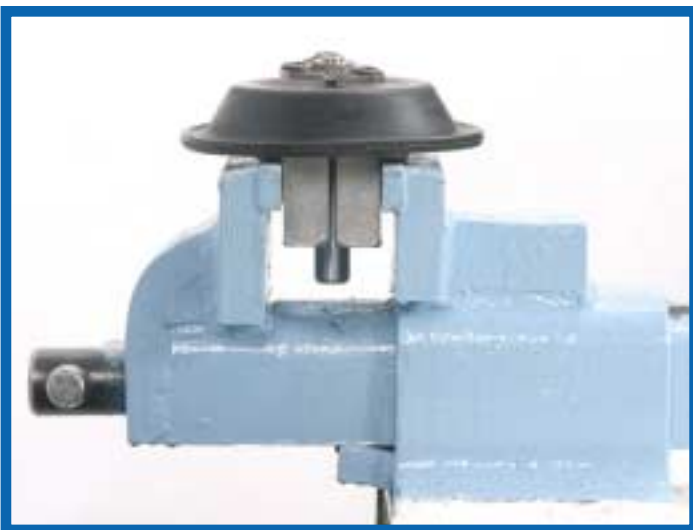
24. Using the wooden block supports (TK SJ) and the AP spanner (APSPANNER) remove the flip flop phantom assembly (APFFASS) of the diaphragm (APDIA) and the diaphragm plate (APDPLT).
