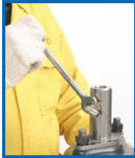
15. With the No. 16 wrench loosen the push fitting (AP1410E) of the cylinder assembling.
