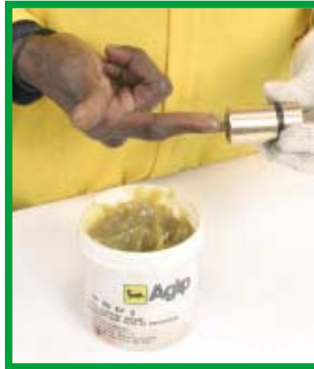
15. Apply lithium based multipurpose grease on the inside and outside the piston guide bush (APGBUSH).
