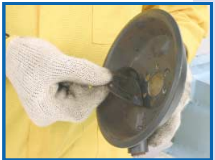
28. Using the No. 5 Allen Key loosen all three flip flop valve screws (AP6X16) of the actuator rear housing (APARH) and remove the exhaust plate (APEPLT), the flip flop body (APFFBOD) and the flip flop valve gasket (APFFVG).
