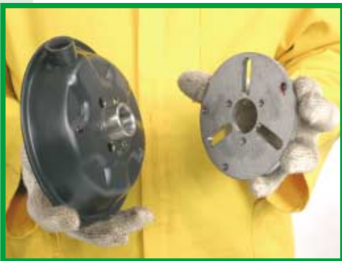
4. Assemble the actuator rear housing (APARH), the flip flop body (APFFBOD), if damaged, a new flip flop valve gasket (APFFVVG) and the exhaust plate (APEPLT) together. Align the set as shown in the red framed picture below.
