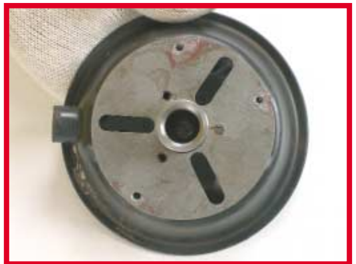
4. Assemble the actuator rear housing (APARH), the flip flop body (APFFBOD), if damaged, a new flip flop valve gasket (APFFVVG) and the exhaust plate (APEPLT) together. Align the set as shown in the red framed picture below.
