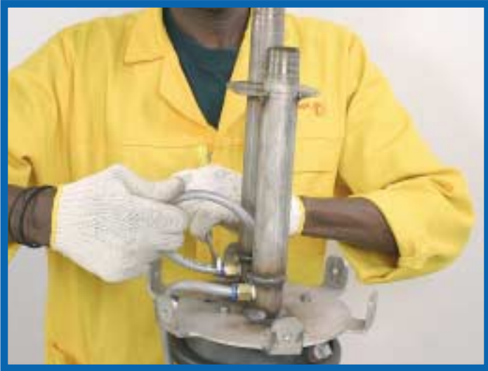
9. Using the No. 11 wrench pull the water and air lines (AP10TU).
