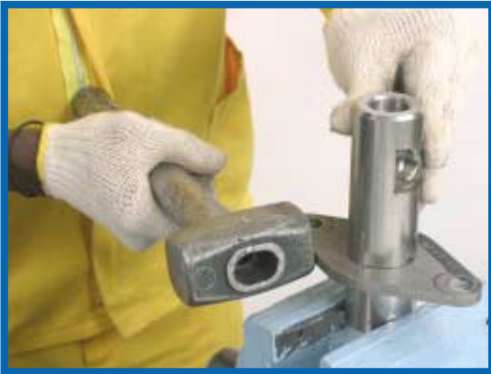
19. Place the cylinder in the bench vise and using the 4 pound hammer remove the cylinder retaining plate (APCRPLT) and the guide bush nut (APBNUT).
