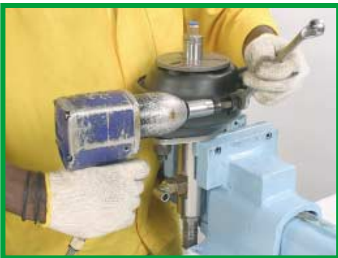
28. Tighten the actuator bolts using No. 14 wrenches and/or pneumatic tool.
