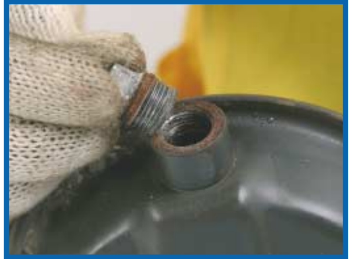
29. Place the actuator rear housing in the bench vise and using the 250mm/10" shifting spanner remove the actuator housing plug (AP38PL).
