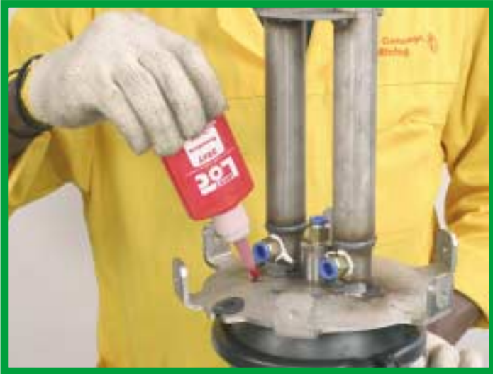
29. Fit the filters assembly, apply threadlock 3247 to the screw holes (AP6X12) and tighten with a No. 5 Allen Key.
