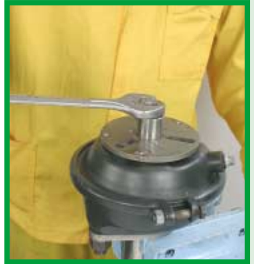
26. Place the actuator in the bench vise with cylinder facing down and put the flip flop cap (APFFCAP) in place, with its corresponding 'O' ring (APFFCO, a new one should there be a leak) and tighten it using a No. 24 wrench.
