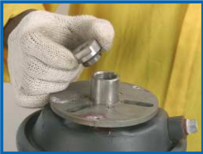
11. Using the No. 17 and 24 wrenches loosen and remove the push on fitting (AP1410S) and the flip flop cap (APFFCAP).
