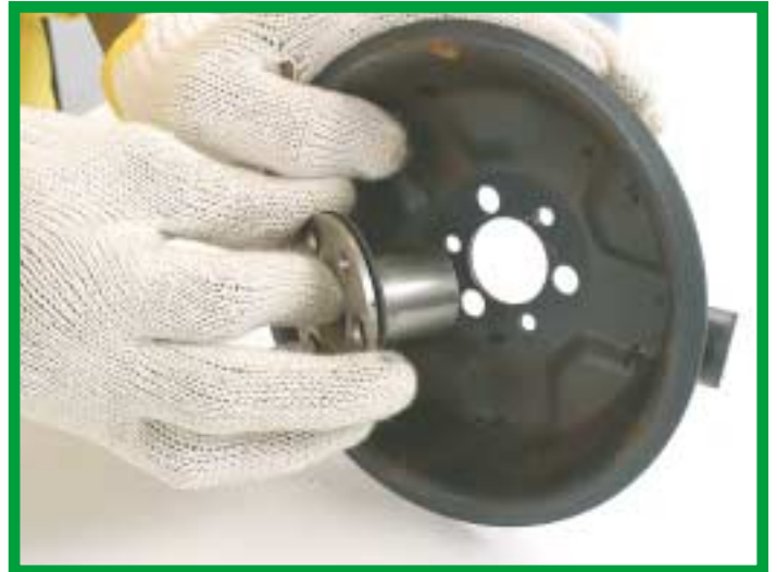
4. Assemble the actuator rear housing (APARH), the flip flop body (APFFBOD), if damaged, a new flip flop valve gasket (APFFVVG) and the exhaust plate (APEPLT) together. Align the set as shown in the red framed picture below.
