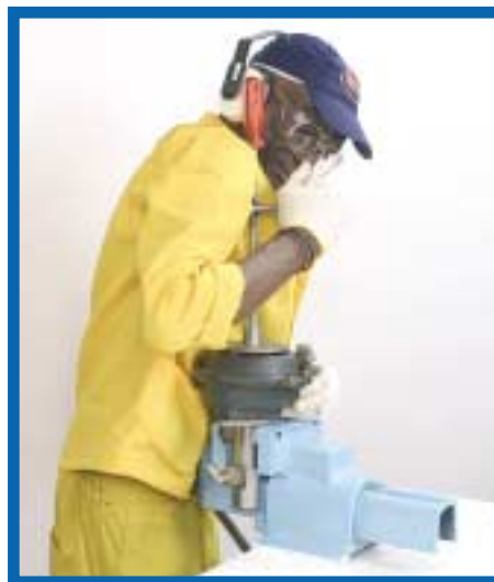
13. Using the 10mm x 300mm screwdriver loosen the popet screw from the flip flop inlet.
