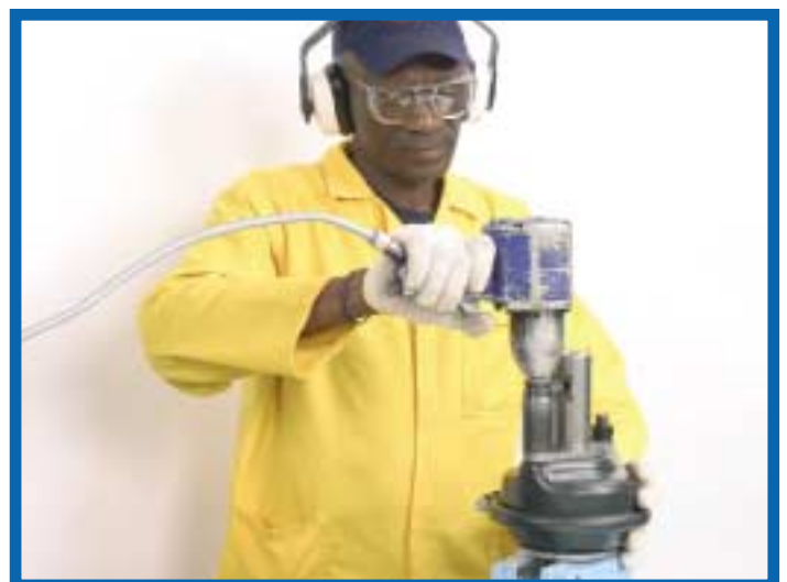
17. Using the pneumatic tool and the No. 24 socket or a No. 24 spanner remove the hexagonal nut (AP16NUT) and the washer (AP16SW).
