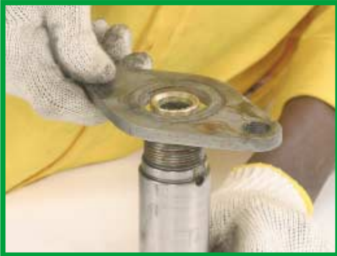
17. Assemble the cylinder (APCYL) with the cylinder plate (APCRPLT) and the guide bush nut (APBNUT).
