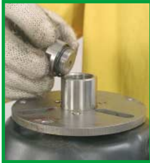
26. Place the actuator in the bench vise with cylinder facing down and put the flip flop cap (APFFCAP) in place, with its corresponding 'O' ring (APFFCO, a new one should there be a leak) and tighten it using a No. 24 wrench.
