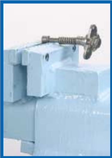
25. Place the flip flop phantom assembly (APFFASS) in the bench vise and using the punch and hammer remove the sellock pin (AP412SP) and disassemble the set.
