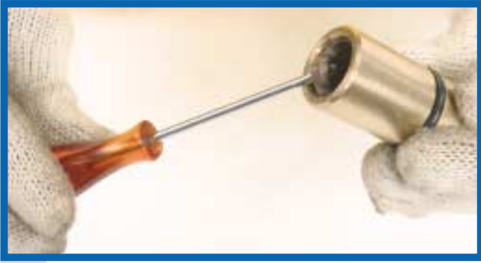
21. Using a small screwdriver remove all the seals and 'O' rings from the inside and outside of the piston guide bush (APGBUSH).
