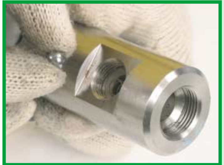
18. Fit the spring (APCVSPR) and the check valve ball (HPBALL) inside the cylinder. If the spring is damaged, it must be replaced.
