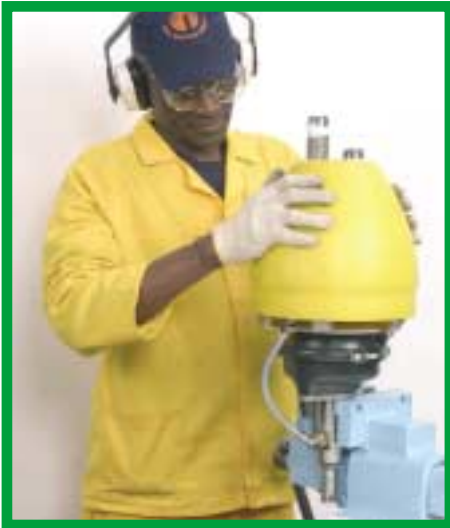
31. Place the pump in the bench vise and assemble the rear housing (APRHOU), the strap (APSTRAP) and tighten the two screws (HP8X16) with the No. 6 Allen Key.
