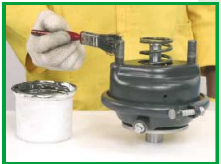
23. Insert the diaphragm spring (APDSPR) into the actuator assembly. Apply lithium based multipurpose grease to the actuator front housing screws and to the piston.
