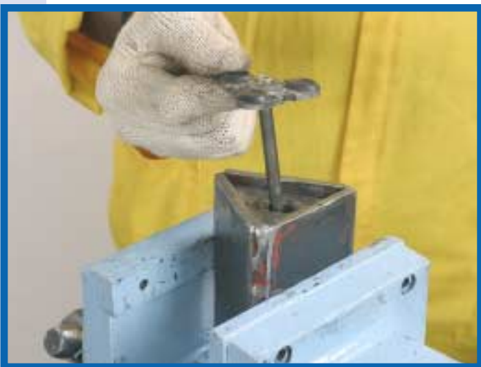
26. Place the flip flop valve plate (APFFVP) and the actuating pin (APAPIN) in the bench vise and using the No.19 wrench loosen the valve's nut (APFFVN).
