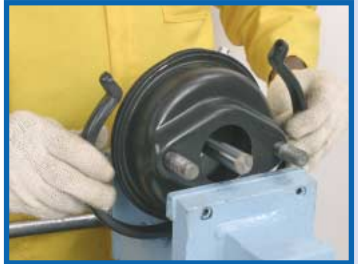
22. Using two No. 14 wrenches or the pneumatic tool with a No. 14 socket, unscrew the actuator housing screw and remove the clamp (APACLP).
