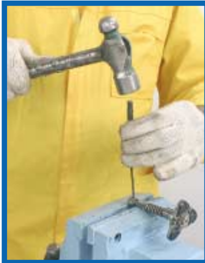
25. Place the flip flop phantom assembly (APFFASS) in the bench vise and using the punch and hammer remove the sellock pin (AP412SP) and disassemble the set.
