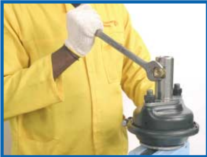
16. With the No. 24 wrench remove the check valve inlet (APCVINL), the Dowety washer (AP12DOW), the ball (HPBALL) and the spring (APCVSPR).
