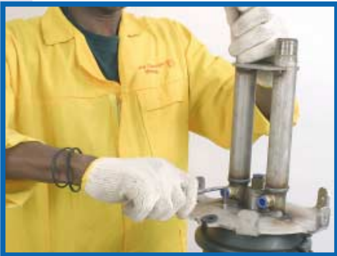
10. With the No. 5 Allen Key loosen the mounting plate screws (AP6X12) and remove the filters.
