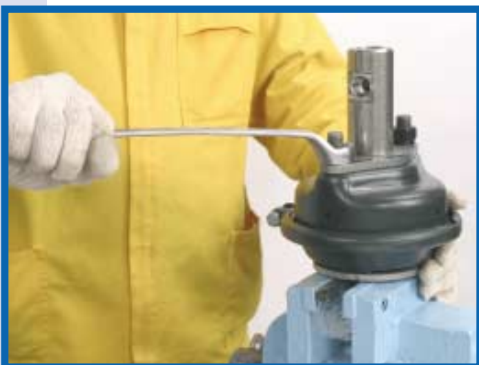
17. Using the pneumatic tool and the No. 24 socket or a No. 24 spanner remove the hexagonal nut (AP16NUT) and the washer (AP16SW).
