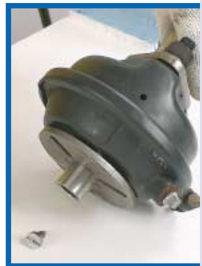
12. With the small screwdriver remove the flip flop cap 'O' ring (APFFCO).
