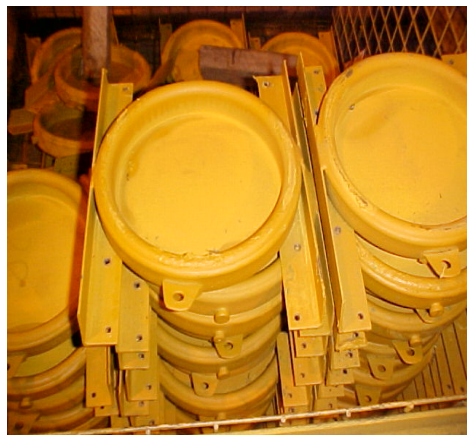
Figure 5 - Jackpots Welded to Angle Frames
